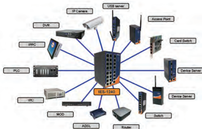
Connections of Ethernet devices
